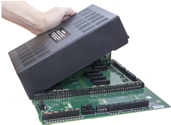
3. Remove the panel module from the protective packaging using adequate electrostatic protection.
