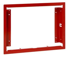
The VES trim ring allows the eVIEW annunciator to easily be recess mounted. VES trim rings provides placement tabs that fold behind dry wall. Traditional screw mounting is available by 2 openings in each of the vertical frames. Conduit entry is not blocked by trim ring.
